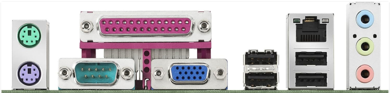
Figure 3: Rear I/O ports of the Intel D425KT Motherboard. This image clearly shows the various connectivity options available at the back of the motherboard, including PS/2 ports, serial ports, VGA, USB, Ethernet, and audio jacks.
