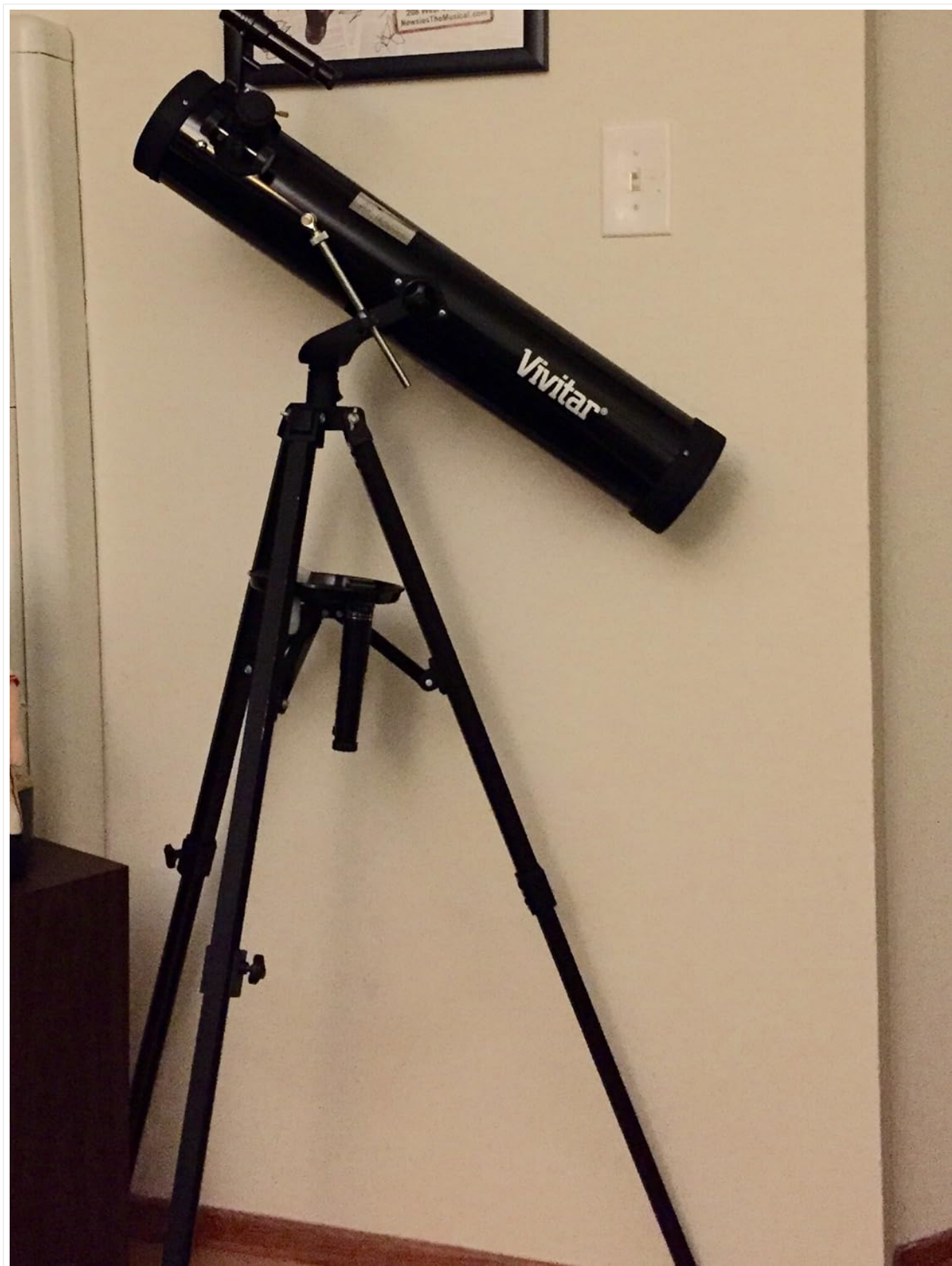
Image: The Vivitar TEL76700 Reflector Telescope fully assembled on its adjustable aluminum tripod, showing the main tube, finderscope, and eyepiece assembly.
