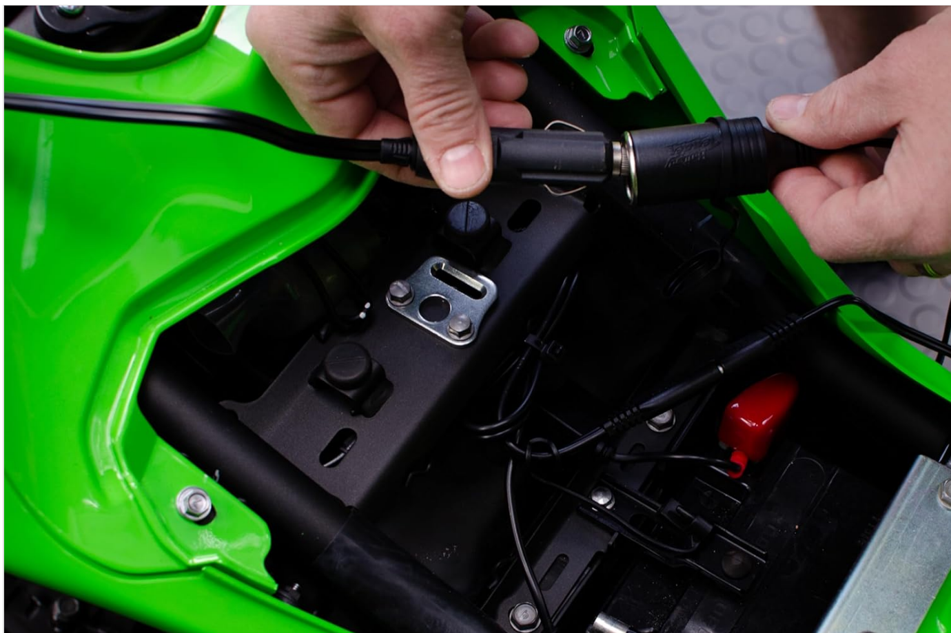
Image: A hand connecting the Battery Tender adapter to an existing battery harness on a motorcycle, illustrating the quick-disconnect feature.
