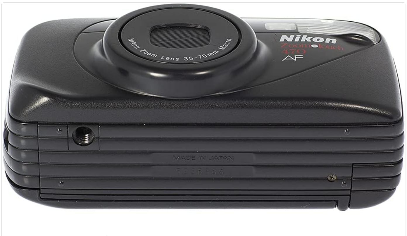
Figure 3.6: Bottom View - Shows the base of the camera, including the tripod socket for mounting on a tripod and the 'MADE IN JAPAN' inscription, indicating its origin.
