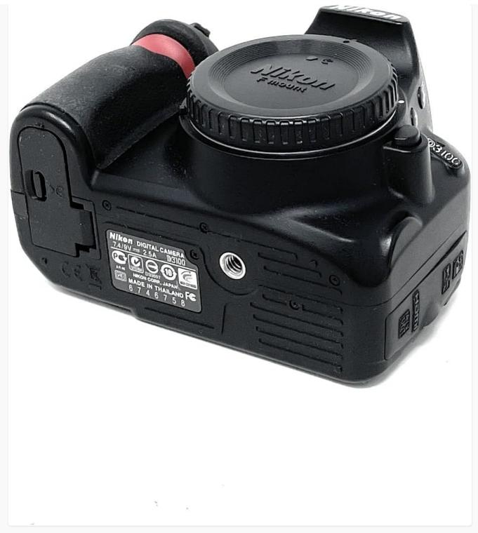
Figure 2.1: Bottom view of the Nikon D3100, showing the battery compartment.
