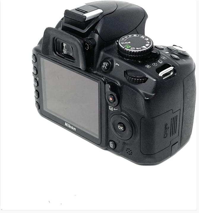
Figure 2.2: Side view of the Nikon D3100, indicating the memory card slot and various ports.
