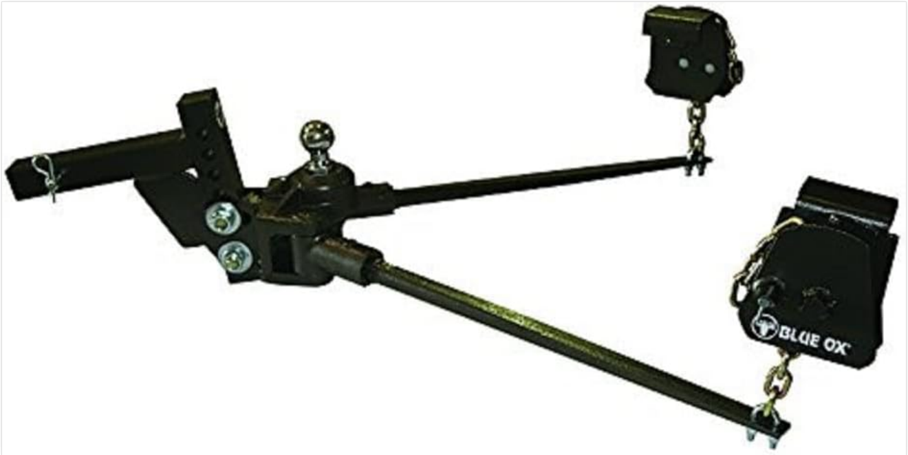
Image 1: Overview of the Blue Ox BXW0750-S Swaypro Weight Distributing Hitch, showing the hitch head, shank, spring bars, and clamp-on brackets.
