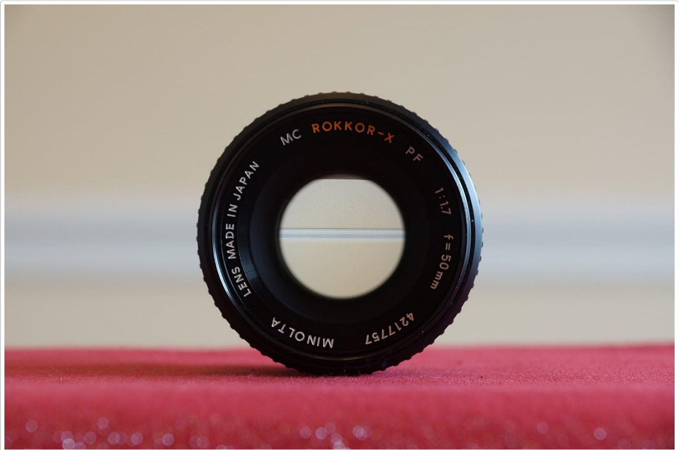
Figure 2.1: Front view of the Minolta MC Rokkor-X PF 1:1.7 F=50mm lens. This image displays the front optical element, the 'MC ROKKOR-X PF' designation, '1:1.7 f=50mm' aperture and focal length, and the serial number '4217757'. The 'LENS MADE IN JAPAN' inscription is also visible.
