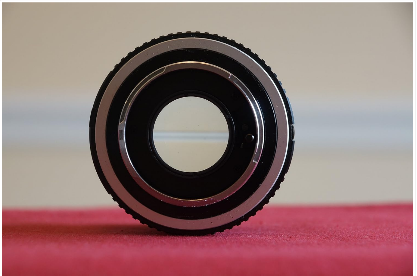
Figure 3.1: Rear view of the Minolta MC Rokkor-X PF 1:1.7 F=50mm lens. This image shows the lens mount, which connects to the camera body, and the rear optical element.
