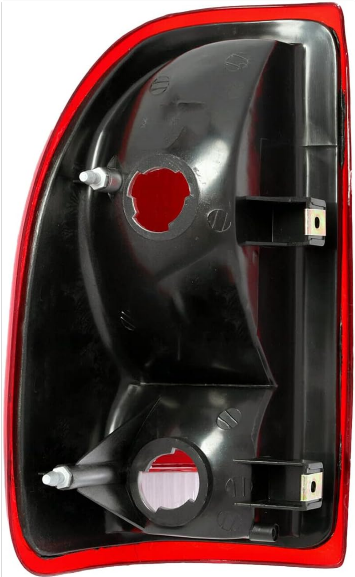
Figure 2: Rear view of the Aftermarket Right Rear Tail Light. This image highlights the mounting studs and the openings for bulb sockets, which are crucial for proper installation and securing the unit to the vehicle.
