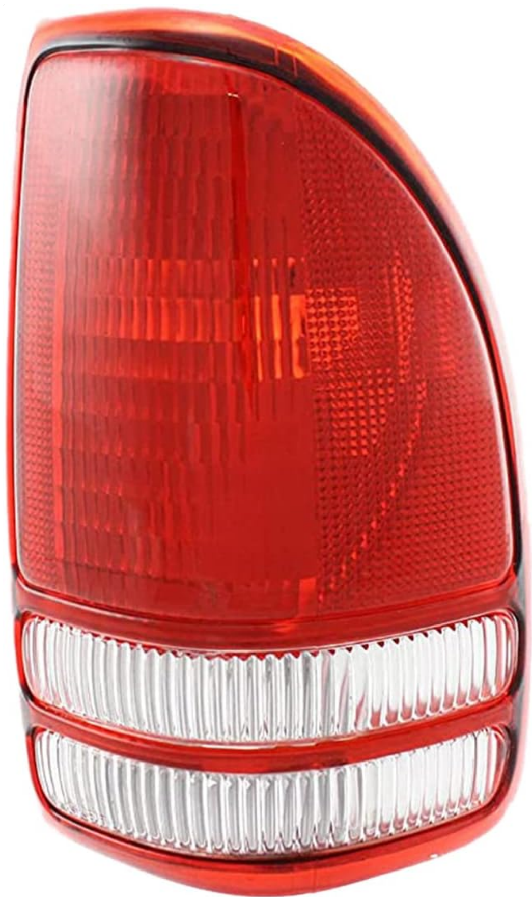
Figure 1: Front view of the Aftermarket Right Rear Tail Light assembly. This image shows the red lens for brake/running lights and clear sections for reverse/turn signals, indicating the external appearance of the unit.
