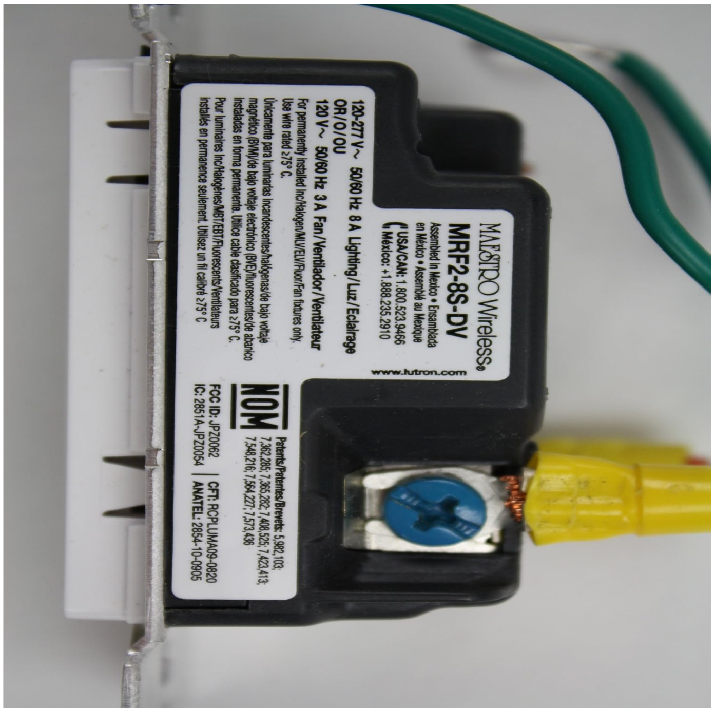
Figure 2: Close-up view of the product label on the back of the Lutron Maestro Wireless Switch, showing model number, electrical ratings (120-277V~, 50/60Hz, 8A Lighting/5.8A Fan), and regulatory information.
