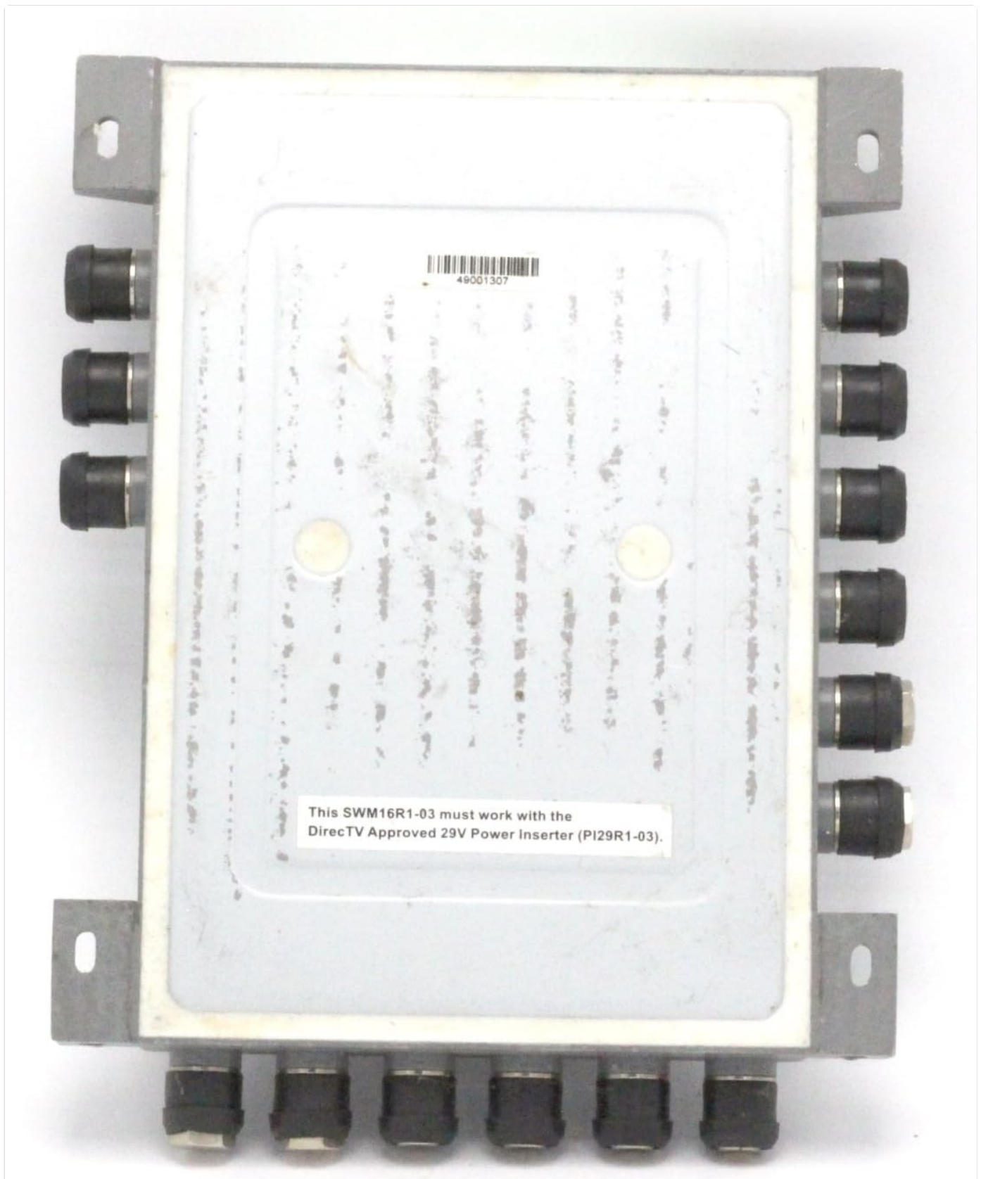
Image: Underside of the SWM16, displaying important compatibility information regarding the required power inserter.
