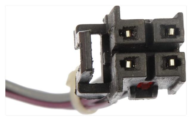
This image shows a detailed view of the multi-pin electrical connector, which is crucial for transmitting fuel level data from the sensor to the vehicle's gauge.
