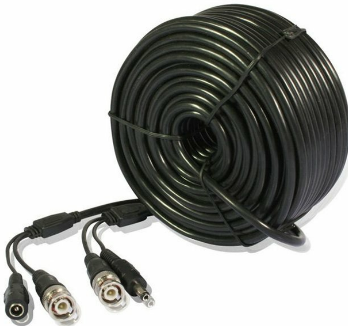
Image: Zmodo W-VPA2030 99-foot pre-made surveillance cable. This image displays the Zmodo W-VPA2030 cable, highlighting its integrated video, power, and audio lines. The cable features BNC connectors for video, RCA connectors for audio, and a 5.5mm barrel connector for power, designed for surveillance camera systems.
