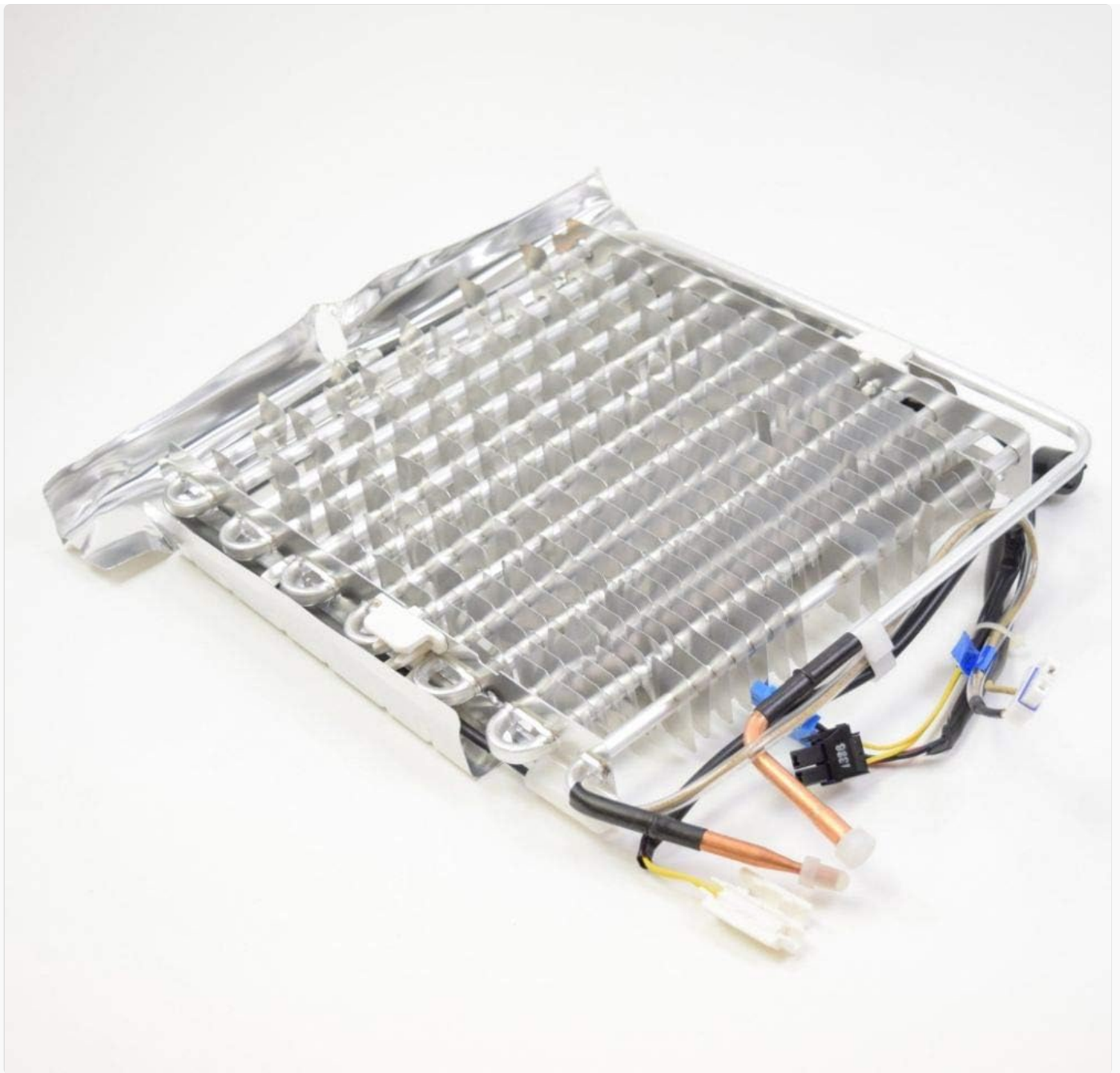
Image 1.1: The Samsung DA96-00762C Refrigerator Evaporator Assembly. This image displays the metallic fins and tubing of the evaporator coil, along with attached wiring and sensors, which are integral to its heat exchange function.
