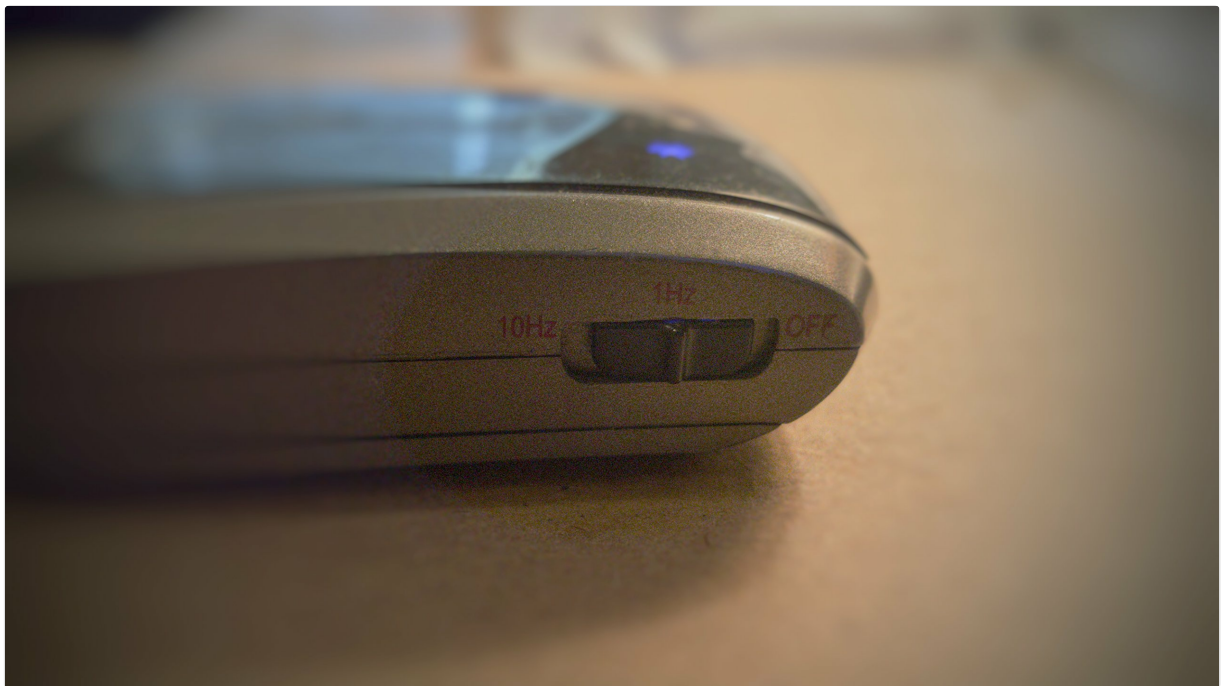
Figure 4.3: Side view of the Qstarz BT-Q818XT, displaying the three-position switch labeled '10Hz', '1Hz', and 'OFF'. This switch controls the GPS update rate and powers the device on or off.
