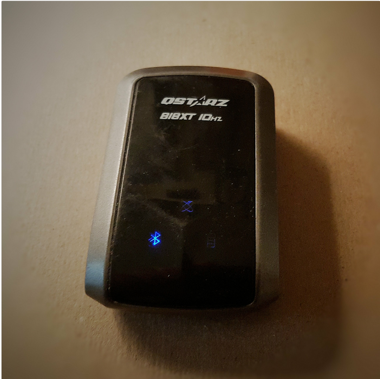
Figure 4.1: Front view of the Qstarz BT-Q818XT receiver. The device features a glossy black top surface with the Qstarz logo and model number '818XT 10Hz' printed on it. A blue Bluetooth indicator light is visible, along with other status indicators.
