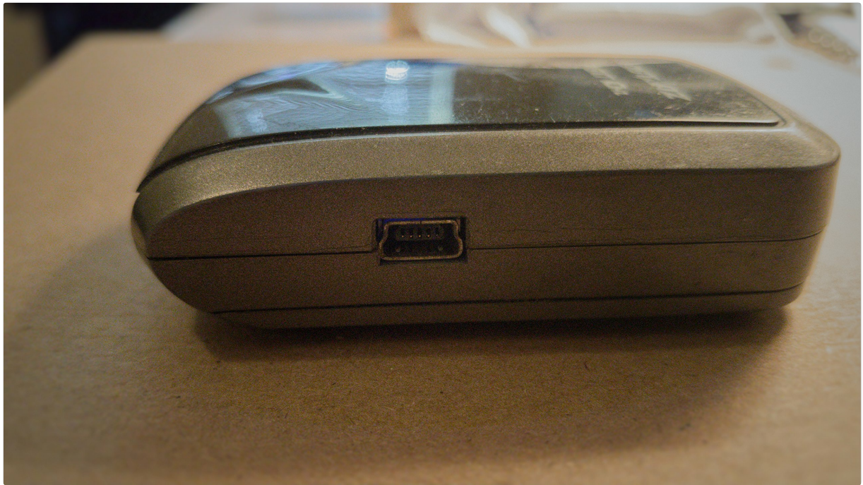
Figure 4.2: Side view of the Qstarz BT-Q818XT, highlighting the Mini USB port. This port is used for charging the device and for connecting it to a computer for use as a wired GPS mouse.
