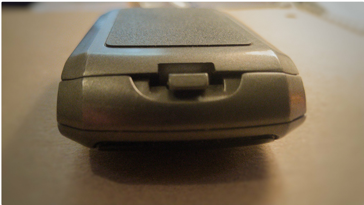
Figure 4.4: Rear view of the Qstarz BT-Q818XT, showing the textured surface and the slot designed for attaching the dashboard mount or other accessories.
