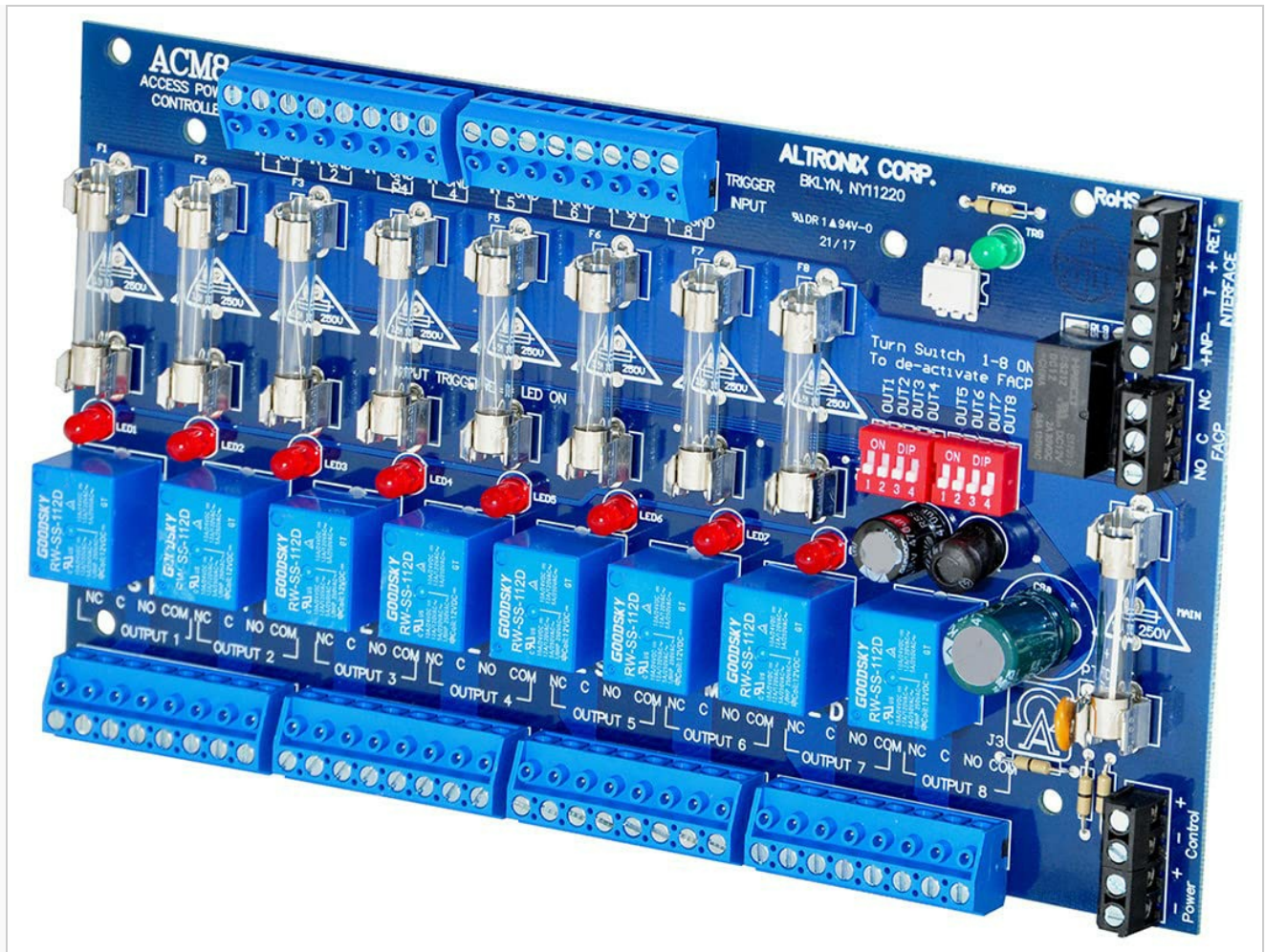
Figure 1: Top-down view of the Altronix ACM8 Access Power Controller board, showing the eight fused outputs, relays, and terminal blocks.
