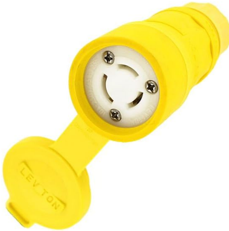
Image: Leviton 25W07 15 Amp, 125 Volt/10A-250V, Locking Blade, Non-Grounding, Wetguard Connector in Yellow.
