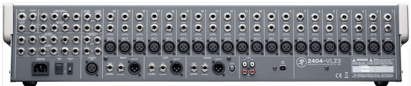
Figure 1: Rear panel connections of the Mackie 2404-VLZ3 mixer. Note the power inlet on the far left.
