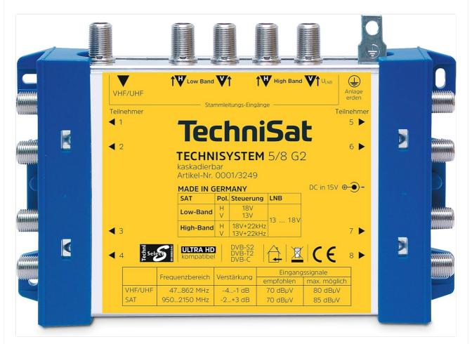
Image 1.1: The TechniSat TechniSystem 5/8 G2 Multi Switch. This image displays the front panel of the multi-switch, showing the input ports for VHF/UHF, Low Band, and High Band satellite signals, along with eight output ports for connecting individual receivers. Technical specifications regarding frequency range and amplification are also visible.
