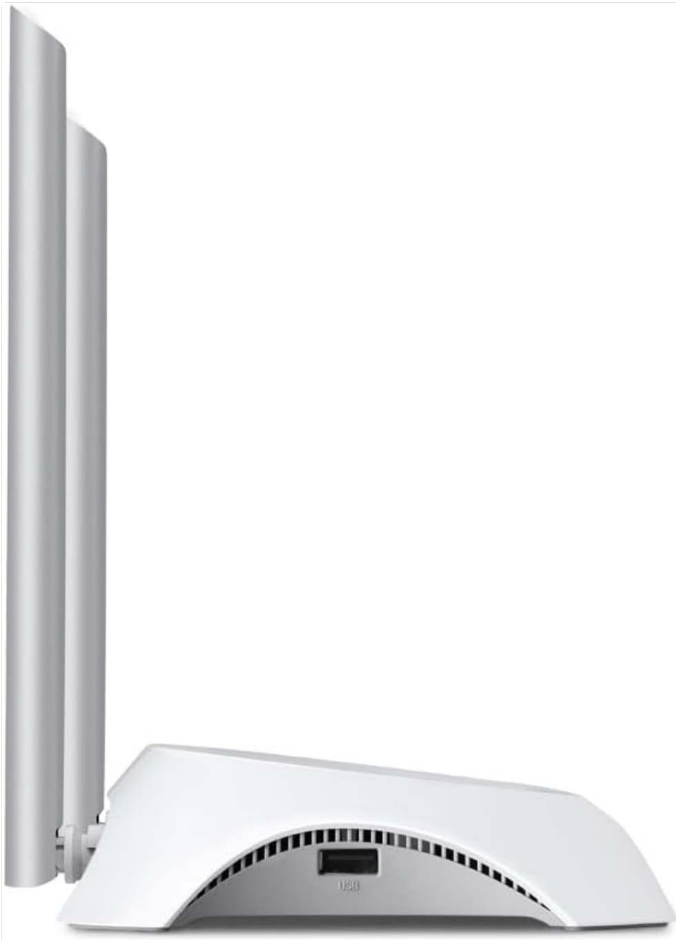
Image: Side view of the TL-MR3420 router, highlighting the USB port for modem connection.
