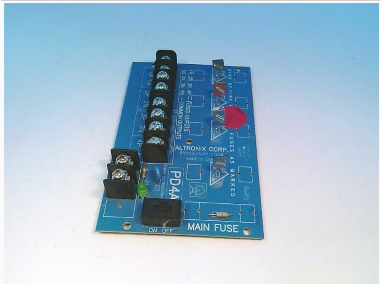
Figure 2: Altronix PD4 Power Distribution Module board, angled view. Highlights the terminal blocks for input and output connections, along with the fuse holders.
