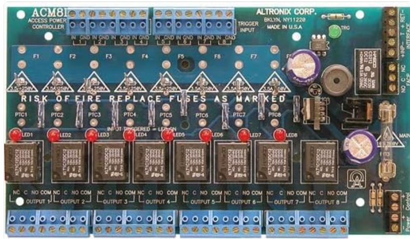
Figure 2: Underside view of the Altronix ACM8CB module, providing a closer look at the circuit board layout and various electronic components, including the PTCs (Positive Temperature Coefficient resettable fuses) and relays.
