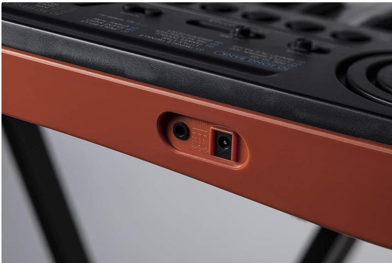
Figure 2: Side view showing the headphone output and DC 9.5V power input jacks.
