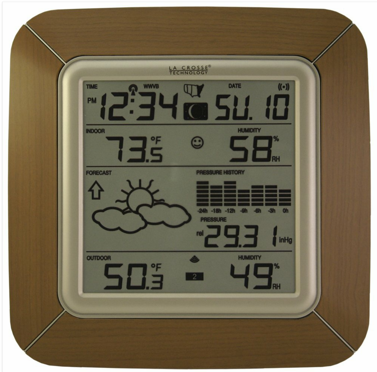
Figure 1: Front view of the La Crosse Technology WS-9057U-IT Forecast Station receiver, displaying time, date, indoor/outdoor temperature, humidity, forecast icons, moon phase, and barometric pressure history.
