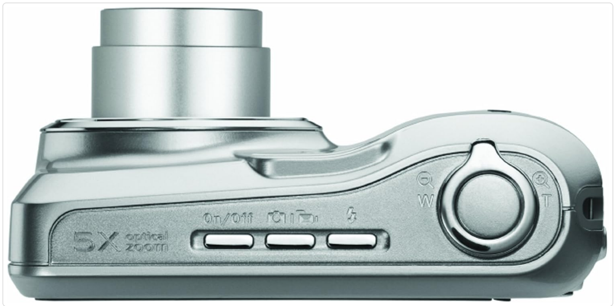
Image: Side view of the Kodak EasyShare C195, indicating the general area for battery and memory card access.
