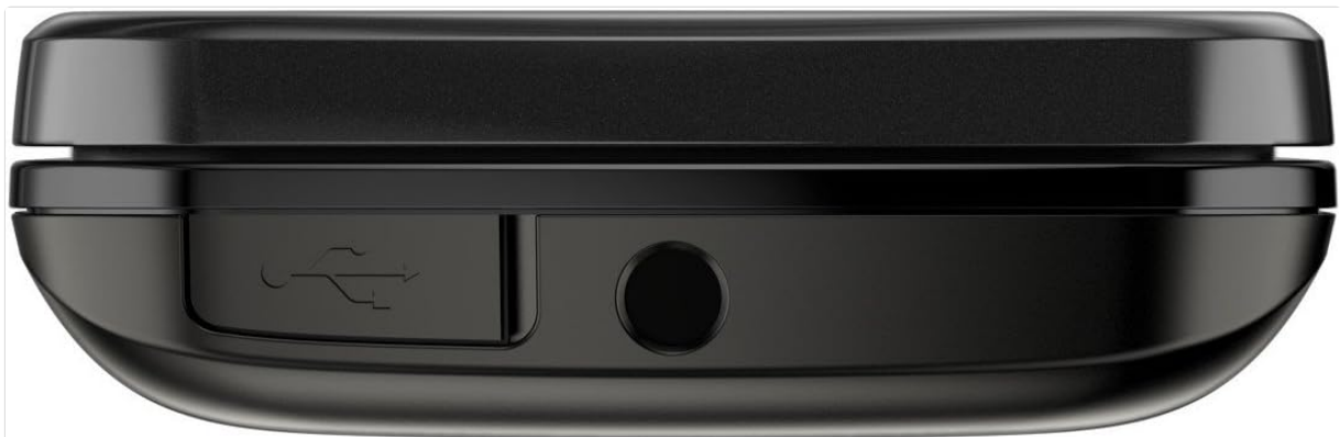
Figure 3.4: Top edge of the Nokia C6, featuring the USB port and 3.5 mm audio jack.
