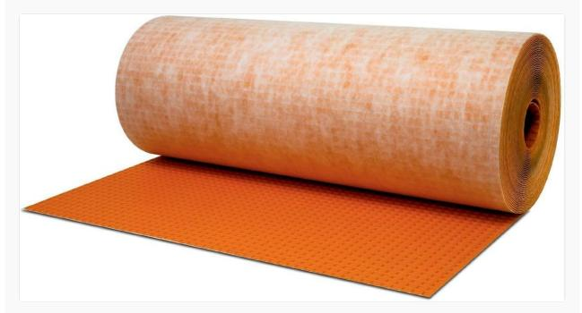
A roll of Schluter DITRA uncoupling and waterproofing membrane. This orange-colored membrane features a waffle-like pattern on one side and a fleece webbing on the other, designed to be embedded in thin-set mortar.
