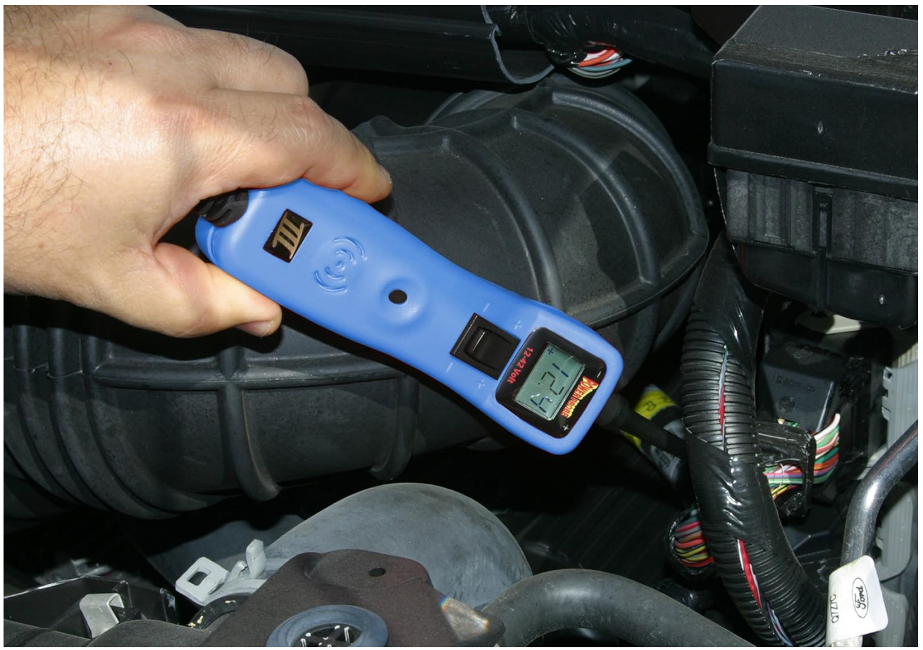
Figure 4: Power Probe III in use, testing an automotive component.
