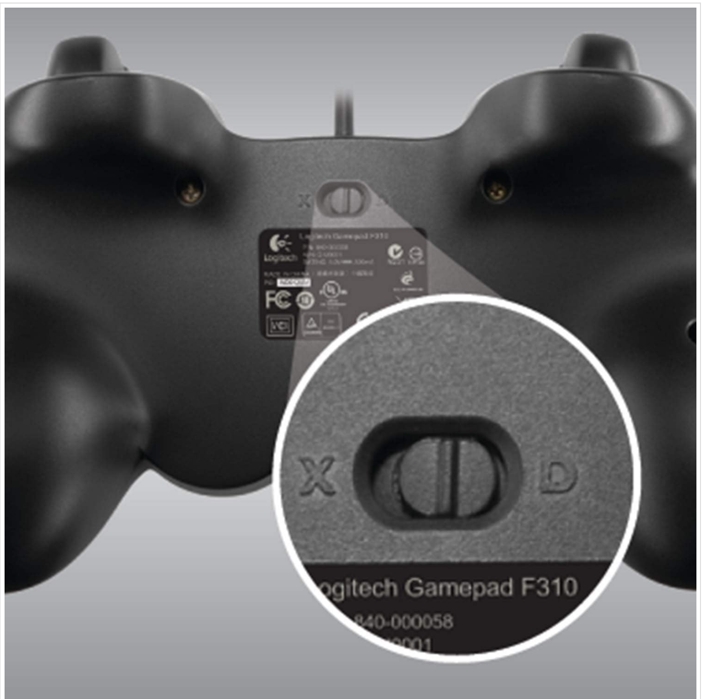
Detail of the X/D mode switch located on the back of the controller, allowing users to toggle between XInput and DirectInput modes for broader game compatibility.
