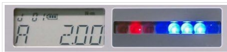
Figure 2: Digital display showing a torque value and visual indicators for reaching the target torque.
