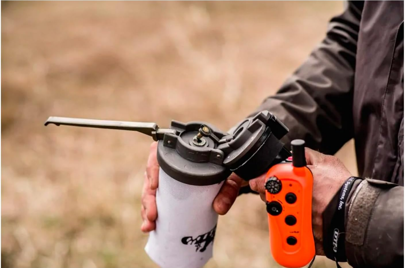
Figure 2: Close-up view of the launcher's firing mechanism and shell extractor.
