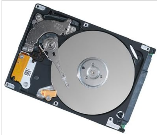
Figure 1: SIB 320GB 2.5" SATA Hard Disk Drive (Internal View)
