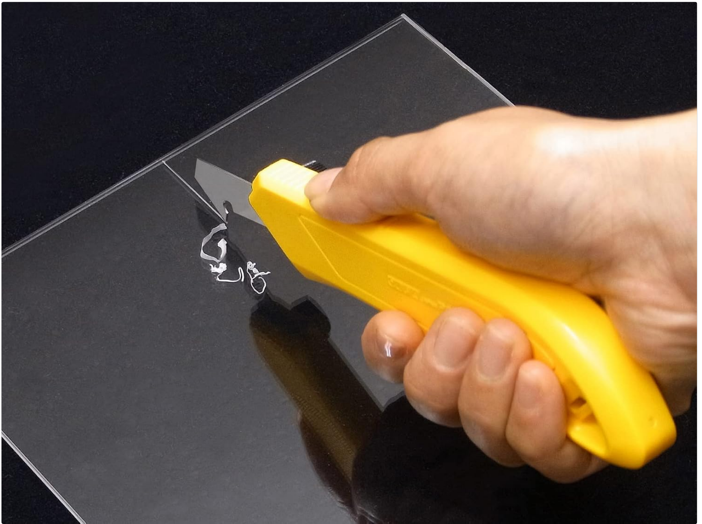
Figure 5.1: Demonstrating the scoring action on a clear plastic sheet.
