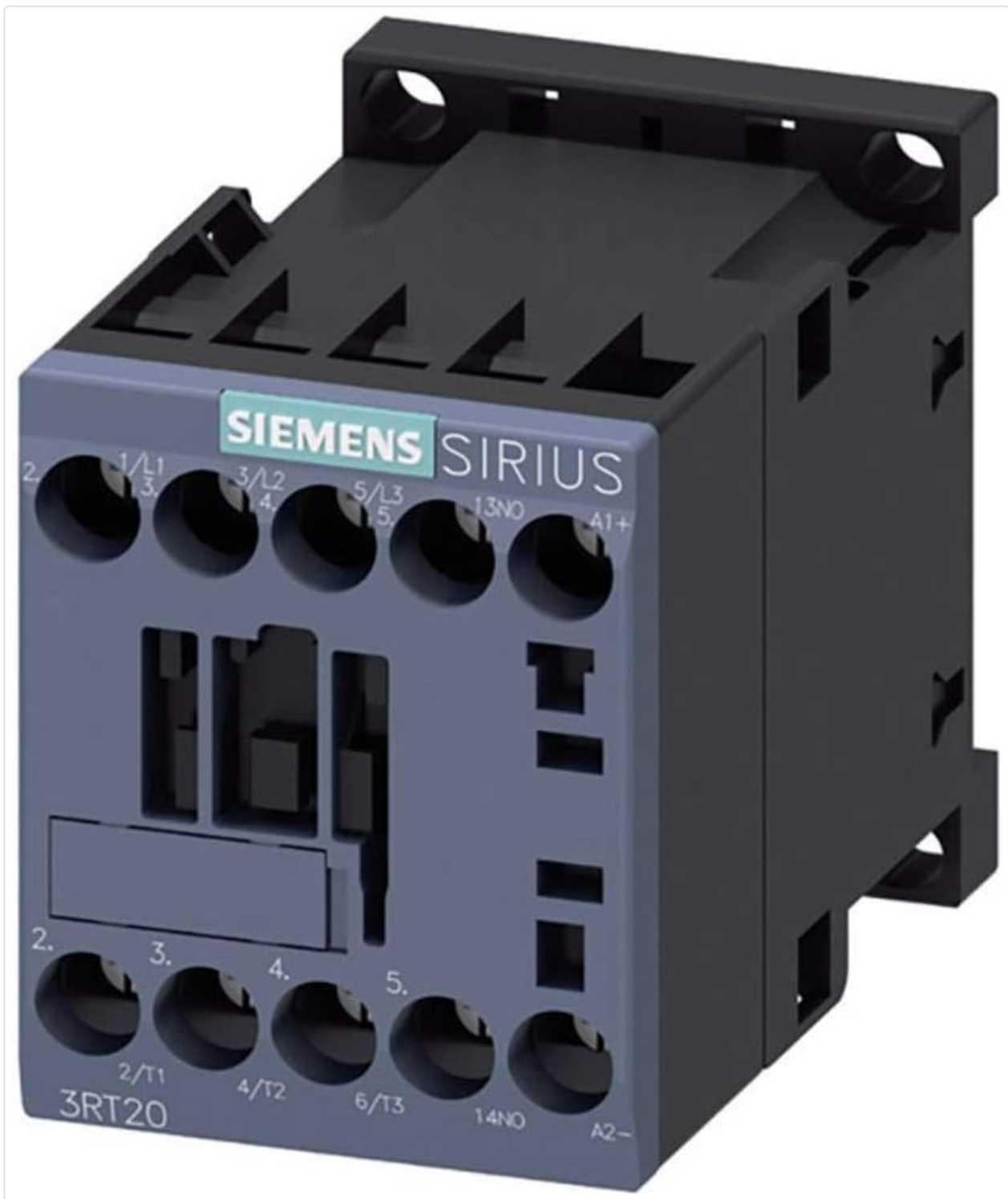
Figure 1: Front view of the Siemens 3RT20151BB41 Contactor, showing main power terminals (1/L1, 3/L2, 5/L3, 2/T1, 4/T2, 6/T3), auxiliary contact (13NO, 14NO), and coil terminals (A1+, A2-).
