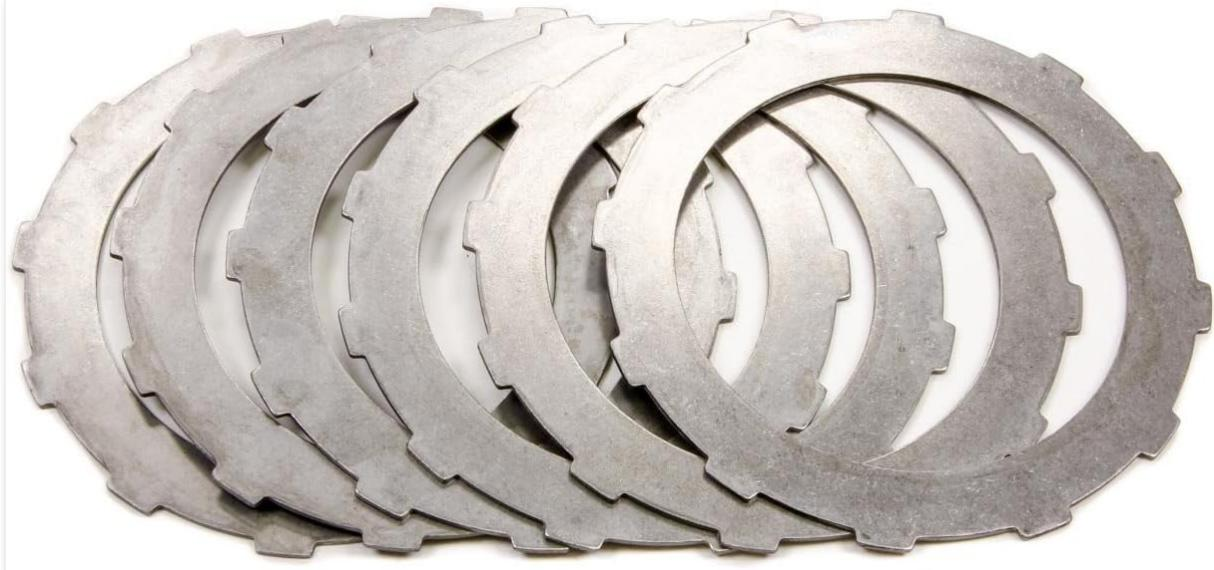
This image displays several TCI 724200 High Gear Steel plates. These are thin, circular metal components, each featuring a series of internal teeth designed for engagement within a transmission system. The plates are stacked or fanned out, showcasing their metallic finish and precise manufacturing.
