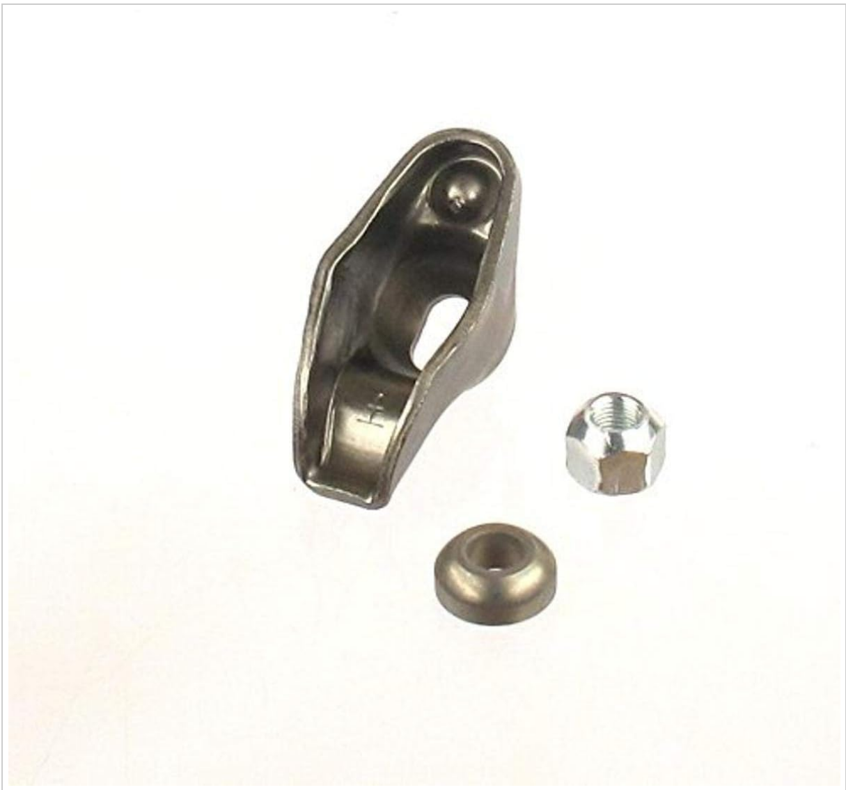
Figure 1: Individual components of the Elgin RK-401 Rocker Arm Kit, including the rocker arm, pivot ball, and adjusting nut.
