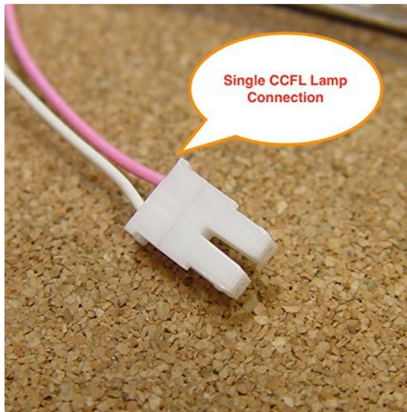
Figure 2.5: Close-up of the single CCFL lamp connection, which powers the backlight.
