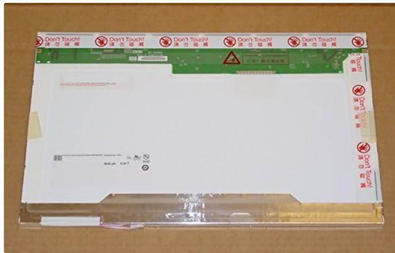
Figure 2.3: Back view of the LCD screen, showing the protective film and integrated circuit board.
