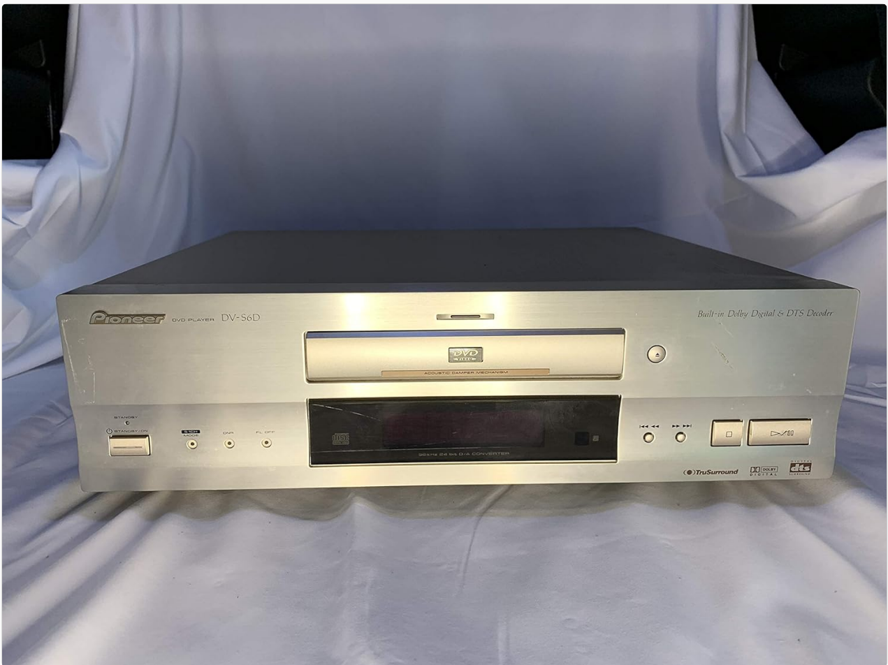
Figure 3.1: Front Panel of the Pioneer DV-S6D DVD Player. This image displays the front panel of the Pioneer DV-S6D DVD Player. The unit features a sleek silver finish. Prominently visible are the disc tray, a digital display, and various control buttons including power, play, stop, pause, and track navigation. The front panel also indicates 'Pioneer DVD PLAYER DV-S6D' and 'Built-in Dolby Digital & DTS Decoder'.
