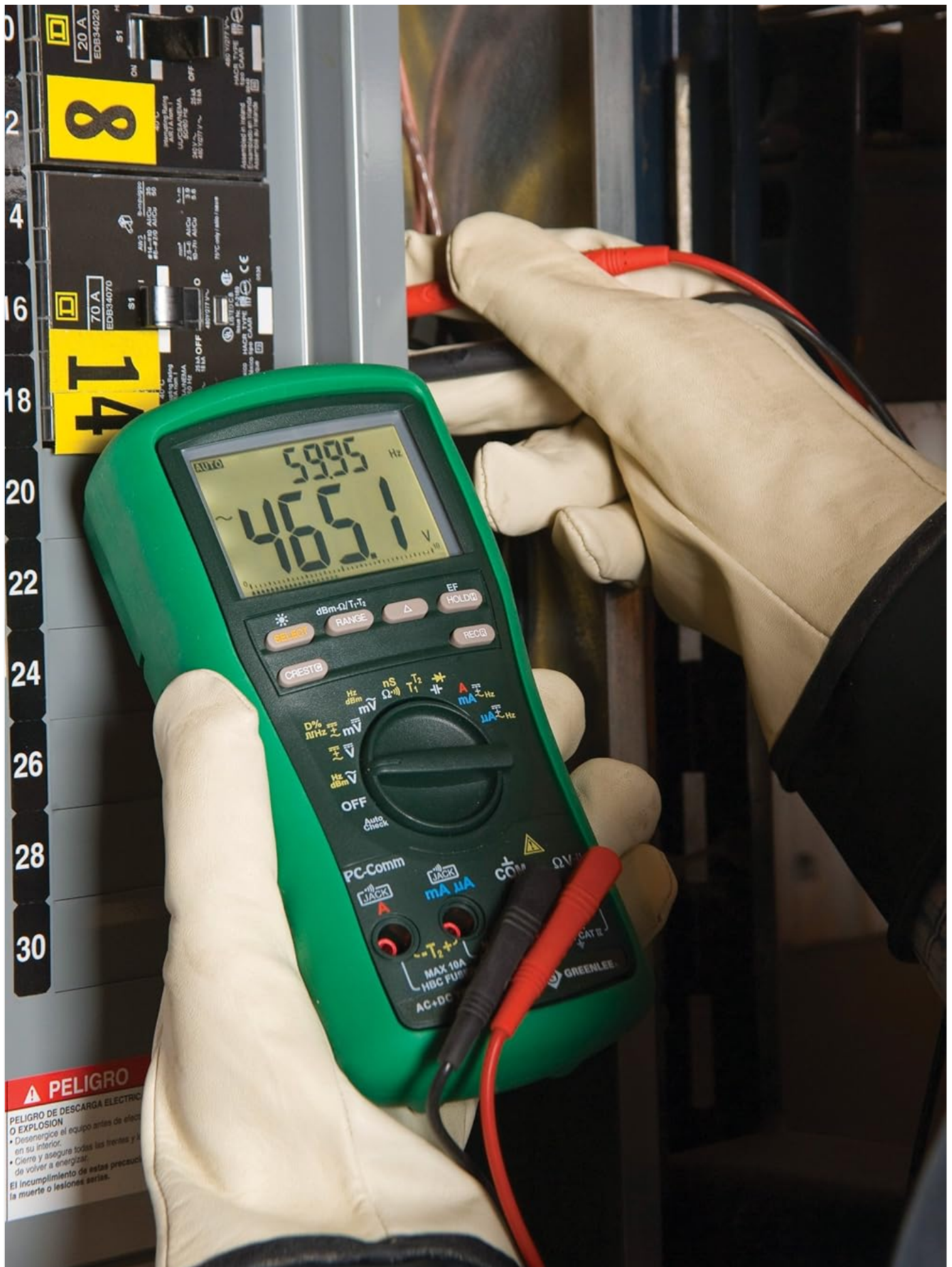
Figure 2: Greenlee DM-830A Digital Multimeter being used to measure voltage in an electrical panel.
