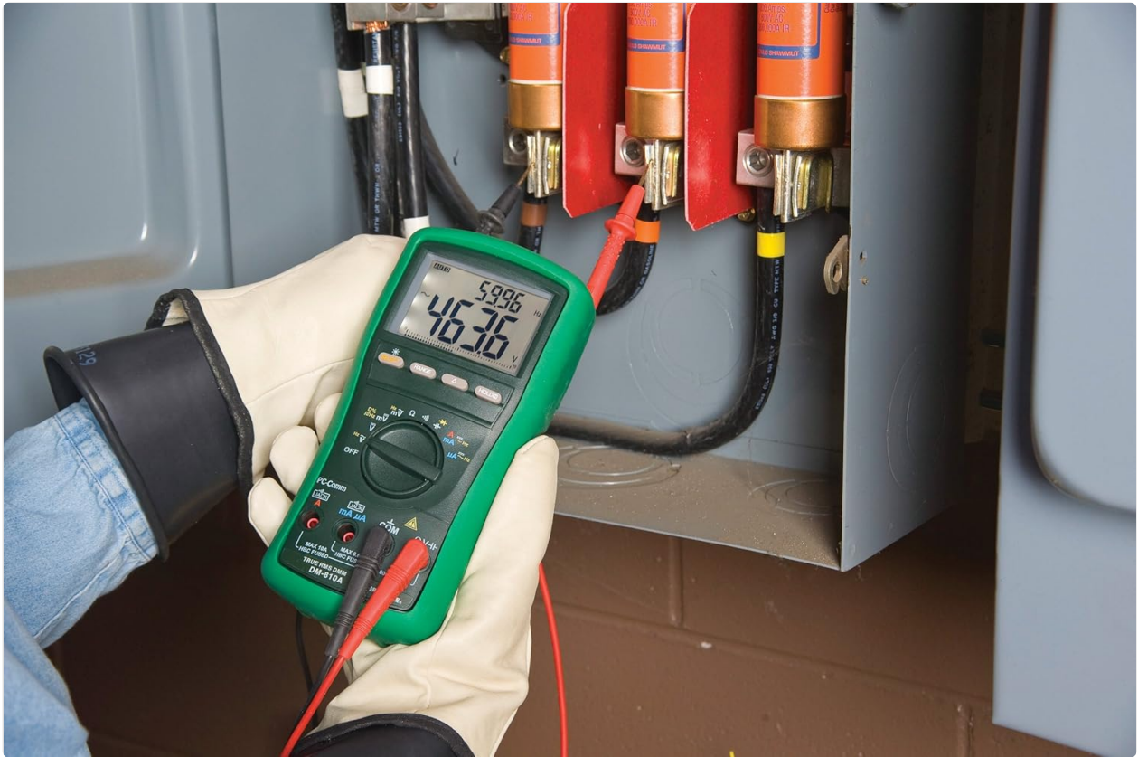
Figure 2: The Greenlee DM-810A Digital Multimeter being used to take measurements within an electrical panel, demonstrating practical application.
