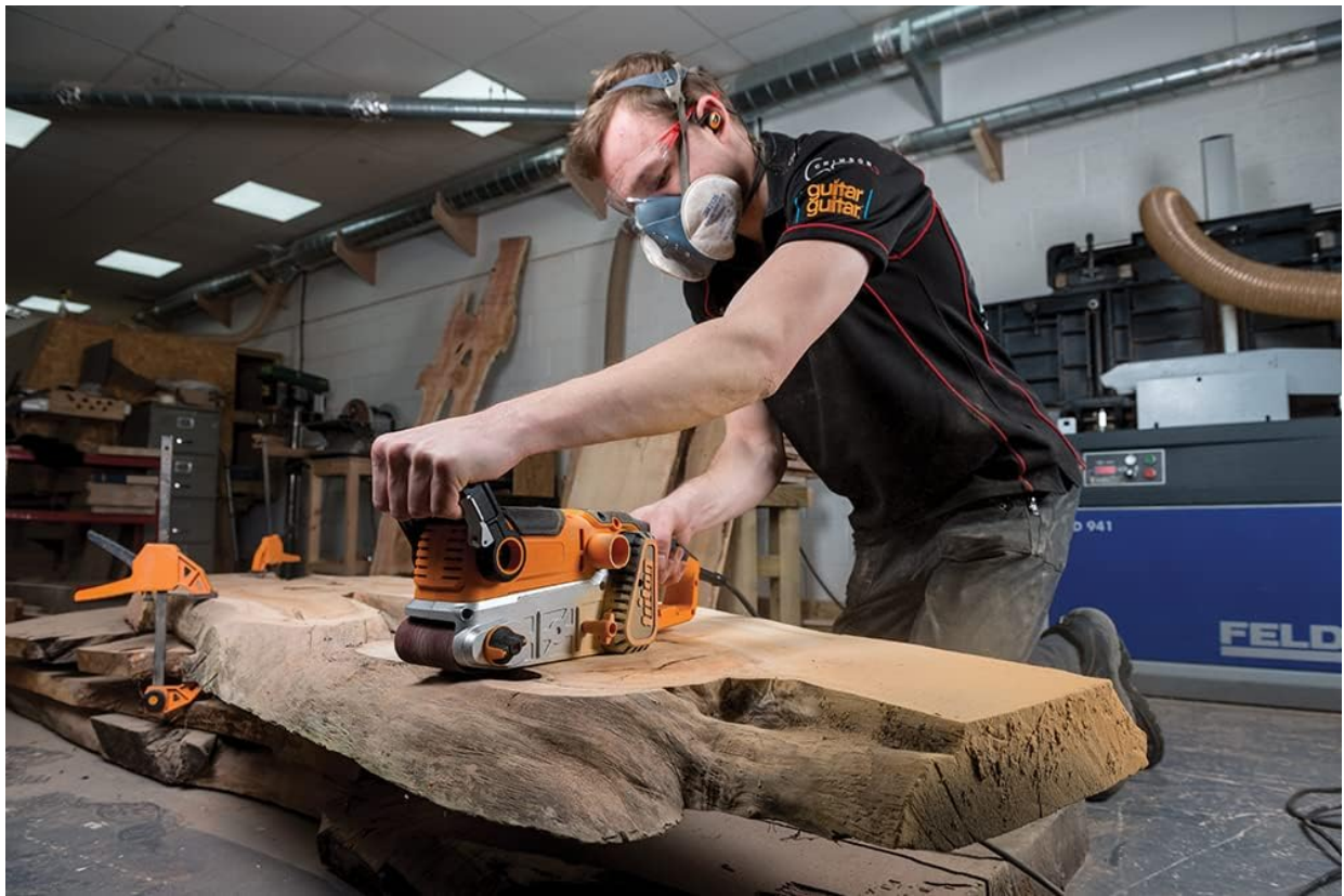
Figure 5.3: A close-up view of the sander in action on a wood slab, illustrating the effective material removal.
