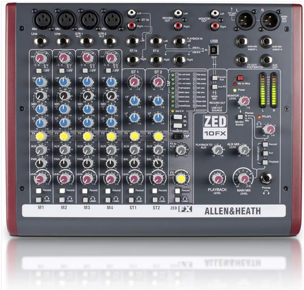
Figure 2.2: Overview of the mixer's top panel with input and output sections.
