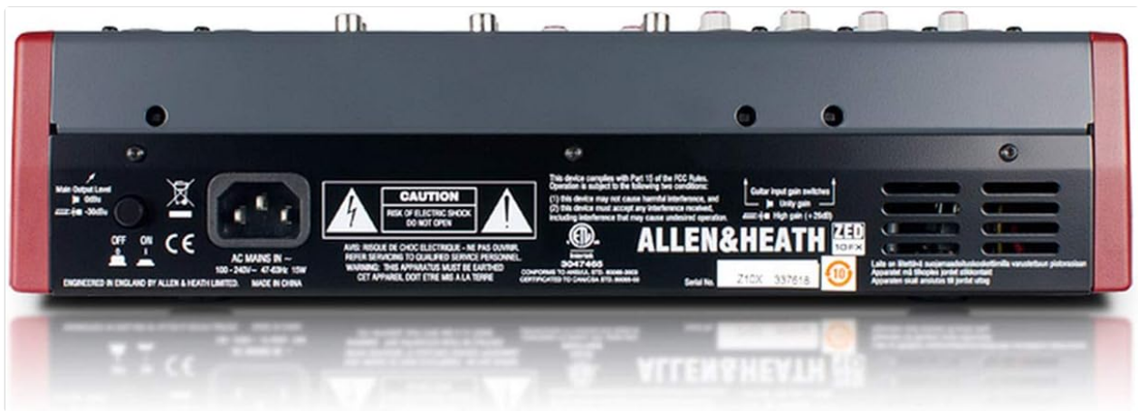
Figure 2.1: Rear panel connections, including the AC mains input.
