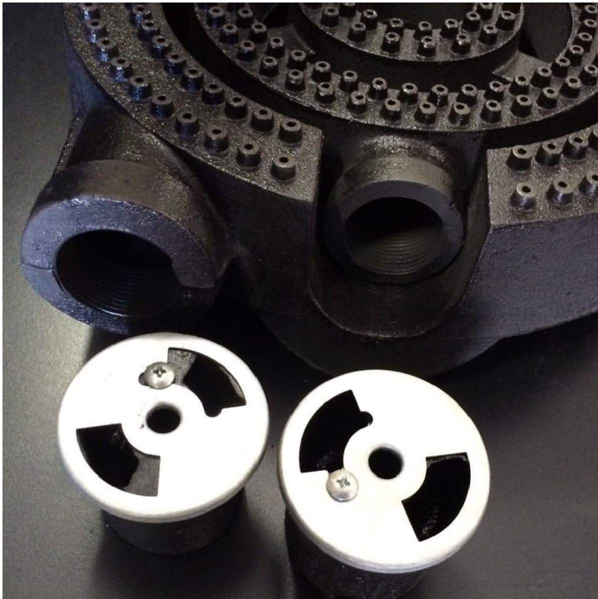
Figure 2: Close-up view of the two air shutters. These components are crucial for regulating the air-to-gas mixture for optimal flame performance.
