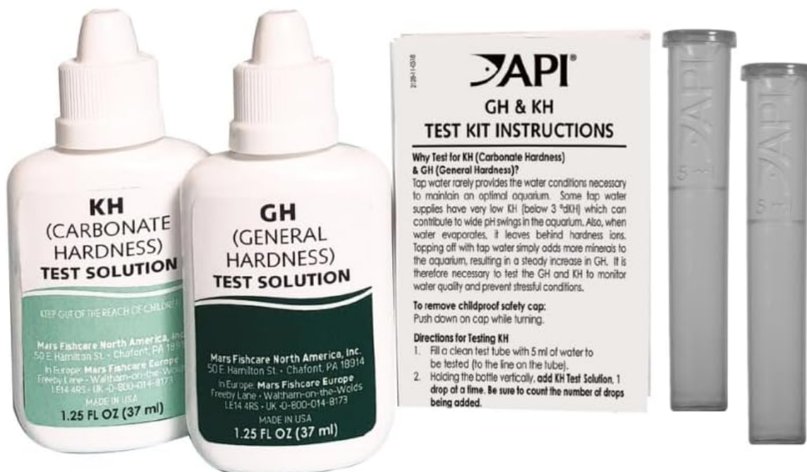
Image 2.1: The complete contents of the API GH & KH Test Kit, including the two test solutions, two test tubes, and the instruction leaflet.
