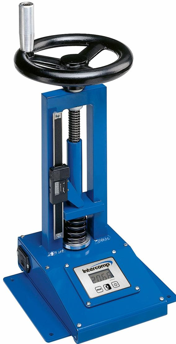
Image: The Intercomp 100058 Valve Spring Tester showing its digital display and the spring compression platform. This image illustrates the overall design and key components of the device, including the handle and base.
