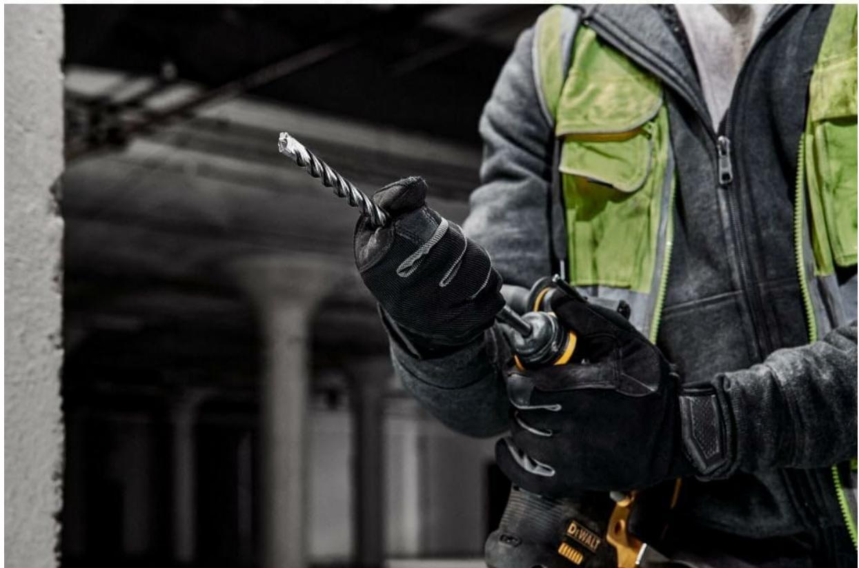
Figure 2: Inspecting the SDS+ drill bit before insertion into the rotary hammer.
