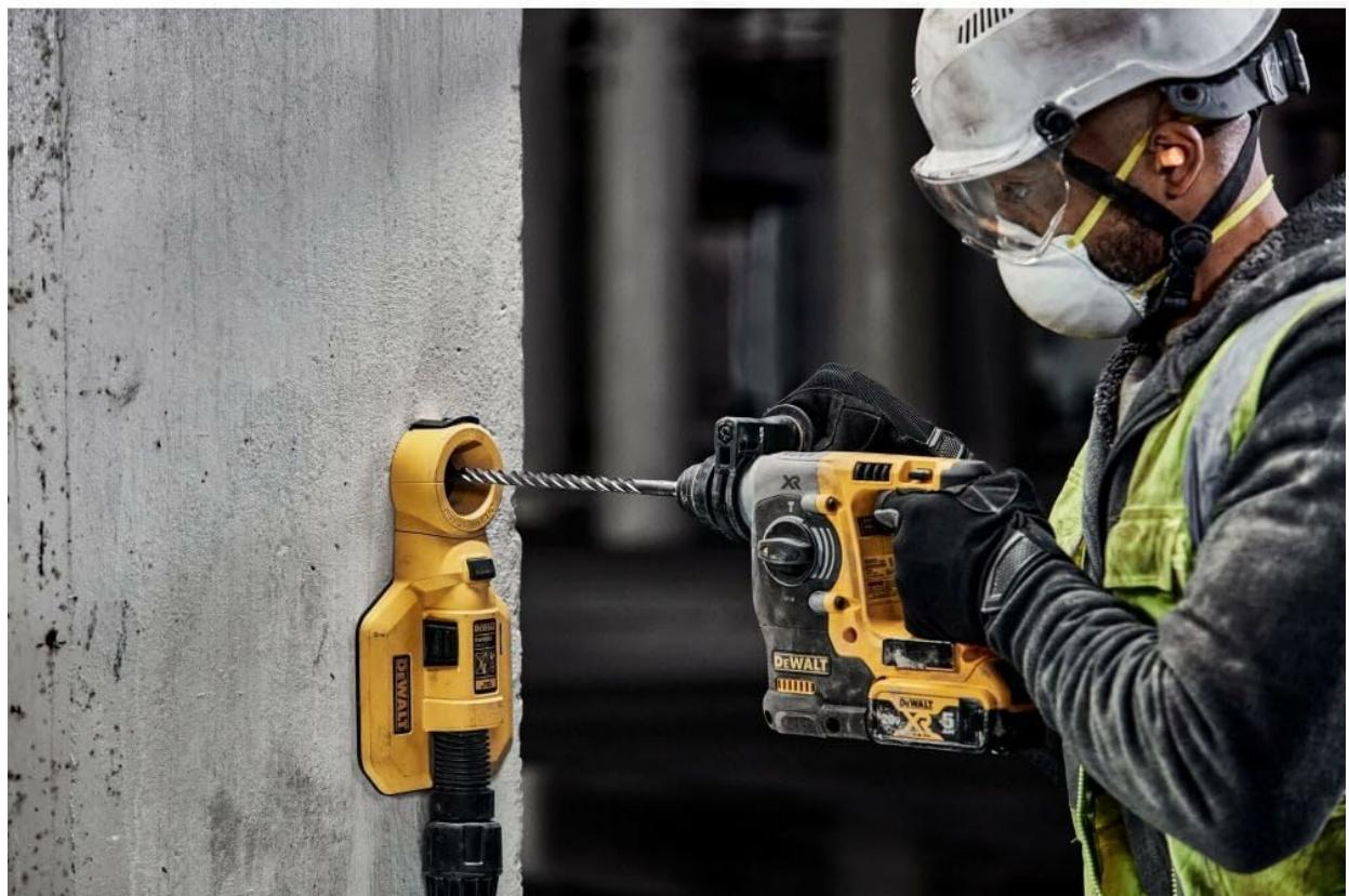
Figure 3: Proper technique for drilling into concrete with the DW5540.
