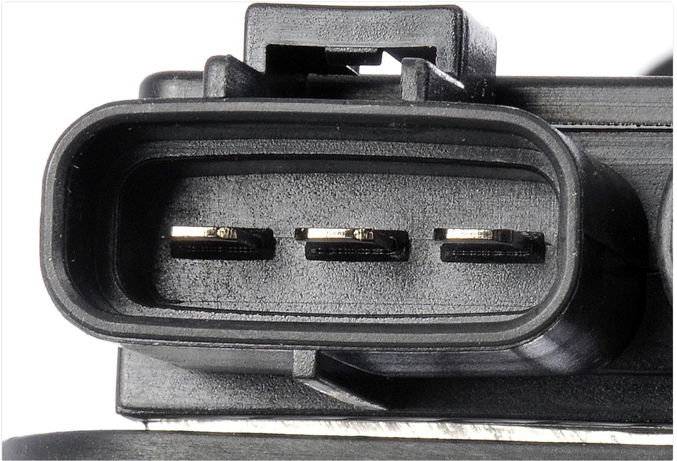
Image 2: A close-up view of the electrical connector on the fan assembly. Ensure this connector is securely attached during installation.
