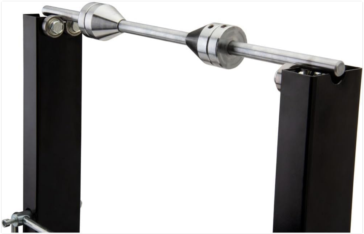
Image: The wheel's shaft properly seated on the stand's rollers.
