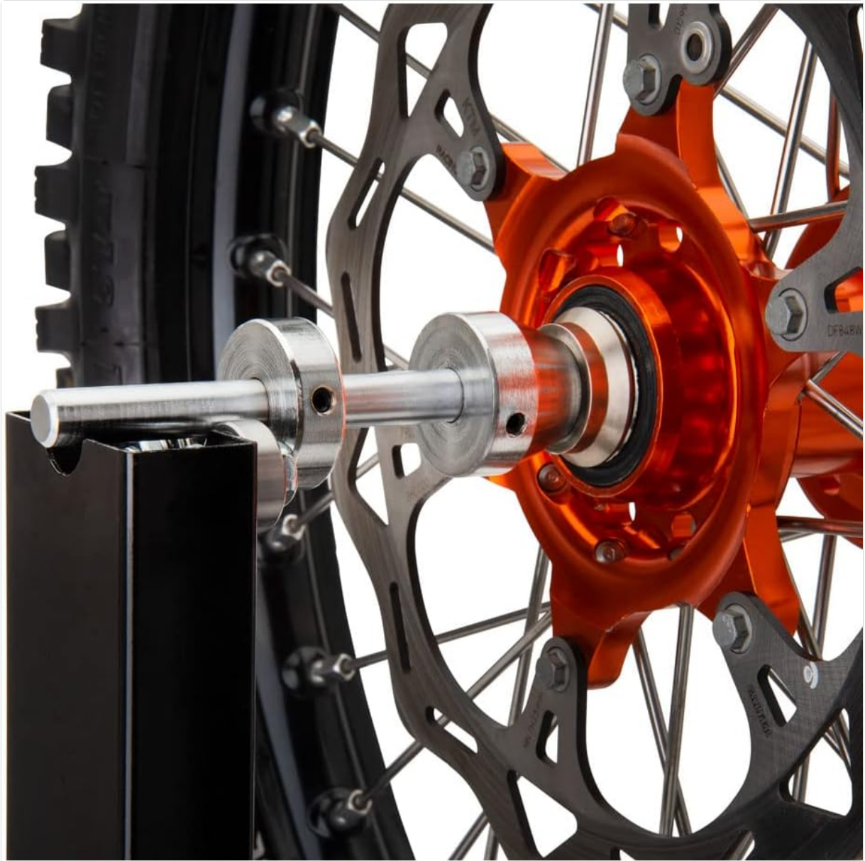
Image: Precision centering shaft with cones securing a wheel hub.
