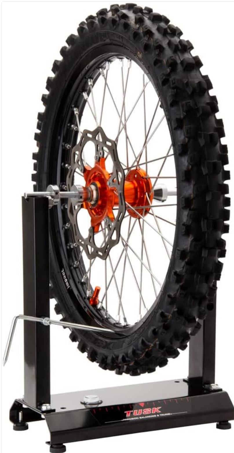
Image: A motorcycle wheel mounted on the stand for balancing.
