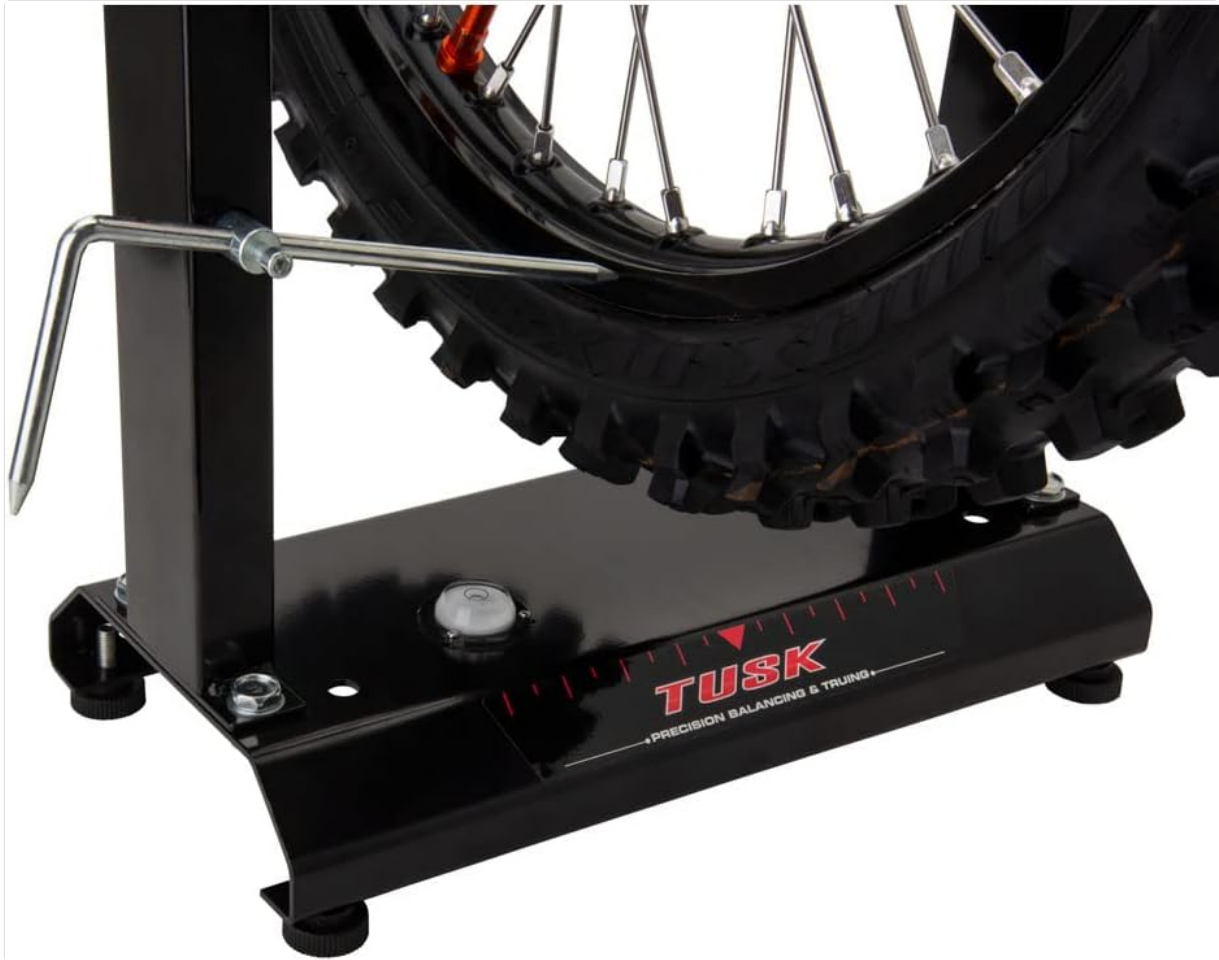
Image: The truing pointer in position to check wheel runout.
