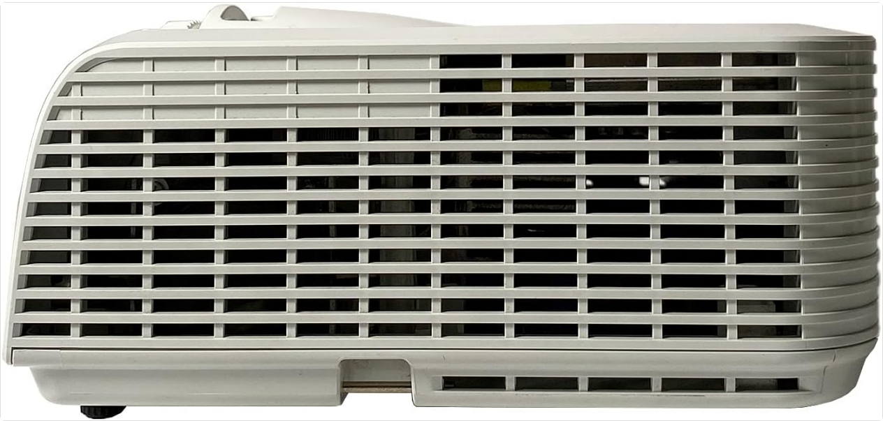
Figure 4: Side view of the Mitsubishi XD280U(D) DLP Projector, illustrating the ventilation grille for airflow. The air filter is typically located behind such grilles.
