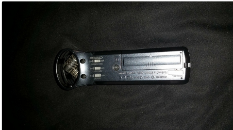
Figure 3: Back view of the Zoom H1, showing the single AA battery compartment, tripod mount, low cut filter, auto level setting, and recording format switches.
