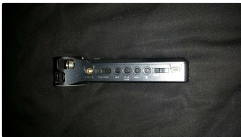
Figure 2: Side view of the Zoom H1, highlighting the transport controls, 1/8 inch external mic input, USB port, and power/hold switch.
