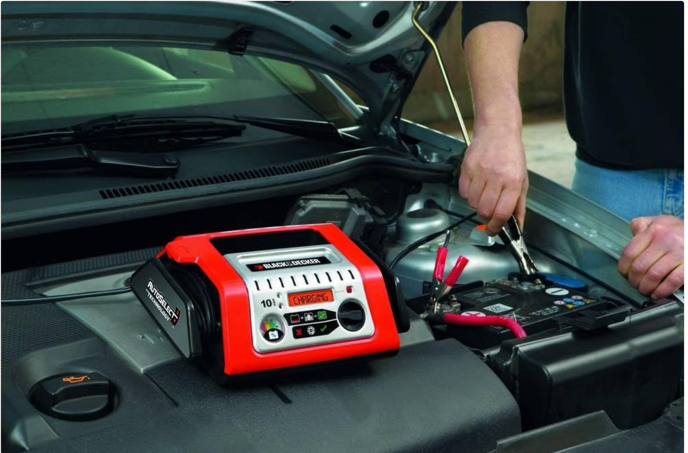
Figure 3.1: Proper connection of the charger clamps to a car battery terminals.
